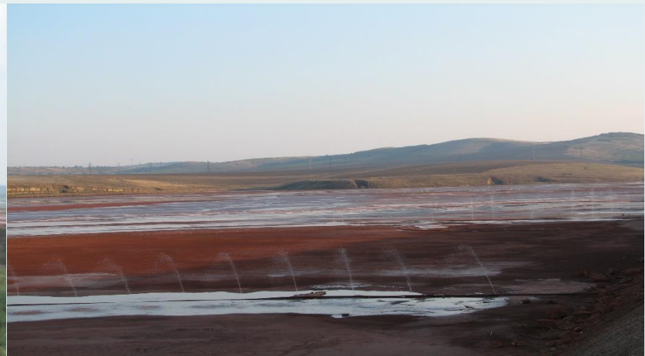
P4. Sprinklers system for spraying the mud surface
